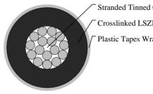
Stranded Tinned Copper Conductor Crosslinked LSZH Insulation Plastic Tapes Wrapping
